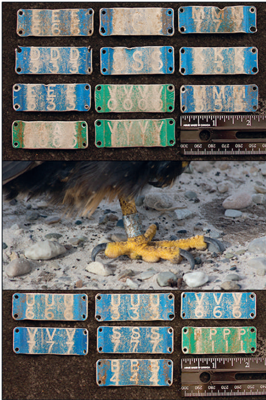
Figure 1. Eleven largely unreadable and seven marginally readable bands removed from caracaras 19–38 mo after being affixed, together with a dirty unreadable worn band on a caracara. (Bands in the figure were flattened by hand and, if necessary with a few taps of a rubber mallet so as to avoid further damage to their surfaces.)
