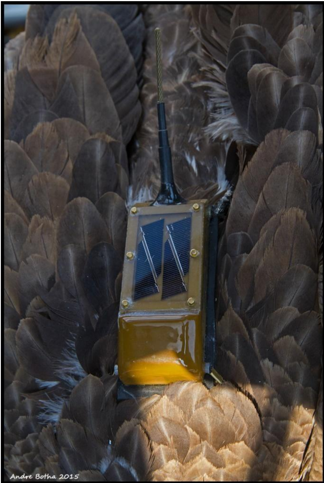
Figure 1.7: Microwave PTT fitted to an African White-backed Vulture. In this instance, the Teflon straps were attached separately to the lugs at the front of the device.
