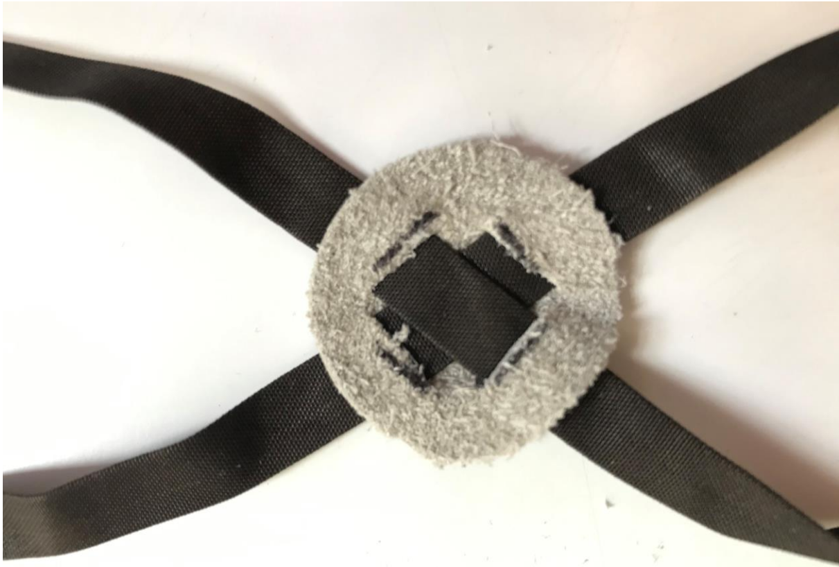
Figure 1.2: Teflon ribbon threaded through the slits cut in the soft leather-hub.
