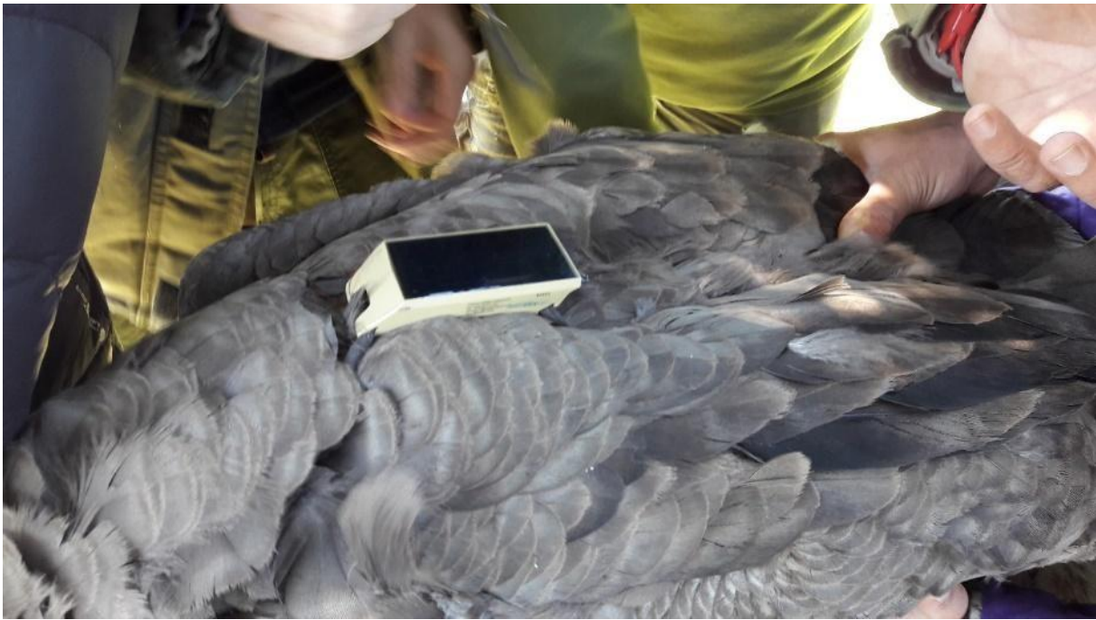
Figure 1.8: Cellular Tracking GPS fitted to an immature Andean Condor. In this instance, the Teflon was attached to the front of the device with a knot in the middle hole.
