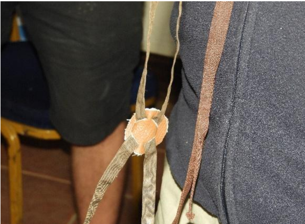
Figure 1.1: Teflon ribbon threaded through the slits cut in the soft leather-hub. The end facing the camera should rest on the bird's sternum when fitted.
